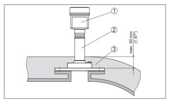
Fig. 23: Mounting the instrument on insulated vessels.
