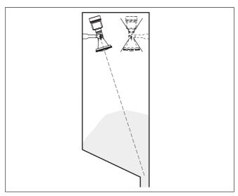
Fig. 25: Installation and orientation in multiple chamber silos
