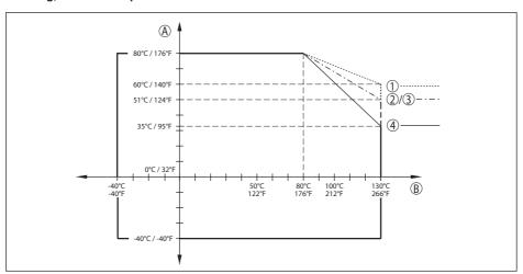
Fig. 54: Derating, ambient temperature, metal-jacketed lens antenna up to +130  $^{\circ}$ C (+266  $^{\circ}$ F)
