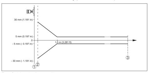
Fig. 53: Deviation under reference conditions
