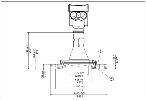
Fig. 70: VEGAPULS 69 with adapter flange DN 100 PN 16
