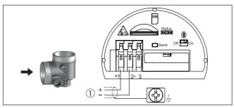
Fig. 34: Connection compartment - Radio module PLICSMOBILE 81
