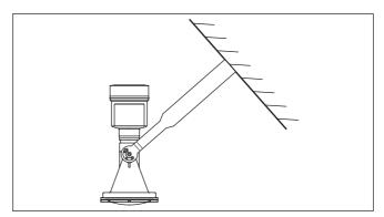
Fig. 5: Wall mounting with inclined wall via the mounting strap with length 300 mm
