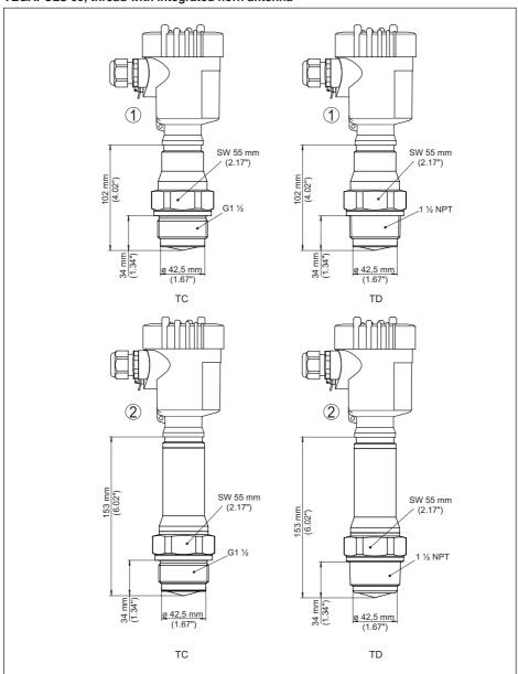
Fig. 73: VEGAPULS 69, thread with integrated horn antenna
