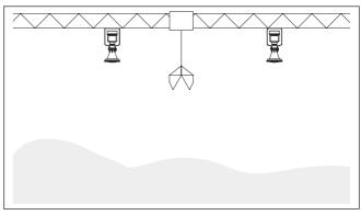
Fig. 22: Radar sensors on traverse crane
