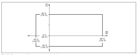
Fig. 56: Derating, ambient temperature, plastic horn antenna
