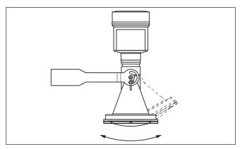
Fig. 9: Adjustment of the angle of inclination
