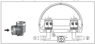
Fig. 33: Terminal compartment, double chamber housing, supplementary electronics " Additional current output"
