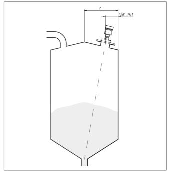
Fig. 18: Mounting position and orientation
