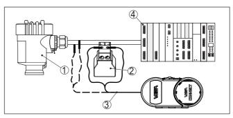
Fig. 49: Connecting the PC via HART to the signal cable
