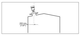
Fig. 12: Mounting the radar sensor on the vessel top
