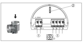
Fig. 38: Electronics compartment - Ex-d double chamber housing
