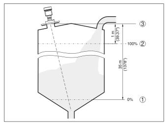
Fig. 47: Parameterisation example, Min./max. adjustment
