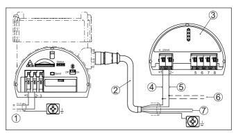
Fig. 37: Connection voltage supply and plics® sensor
